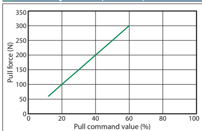
Correlation diagram between pull force and pull command value
